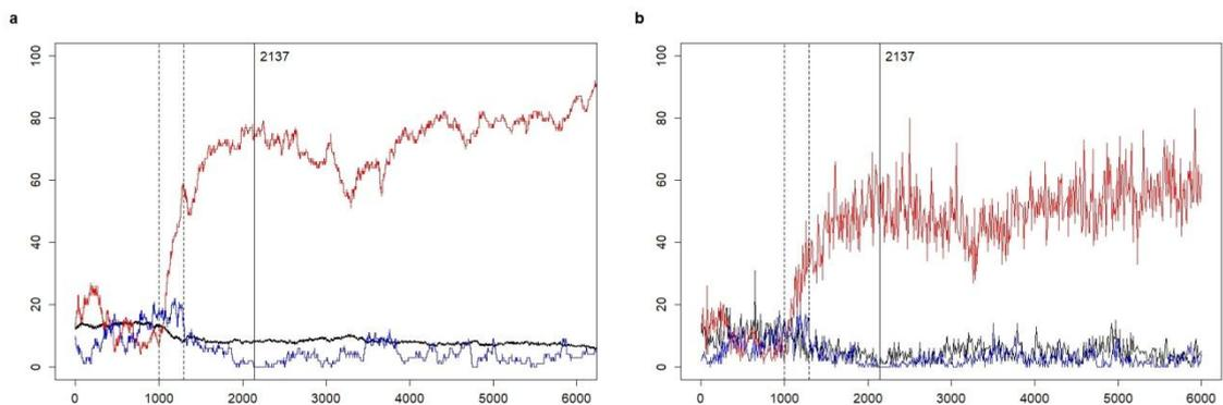
Fig. 7. The same model simulation with stimulus provided by 10 active neurons for 300ms represented by: a) proportion of active neurons in each pool; b) average frequency of spiking neurons in pools A, B and 100 neurons from the rest of the network.
