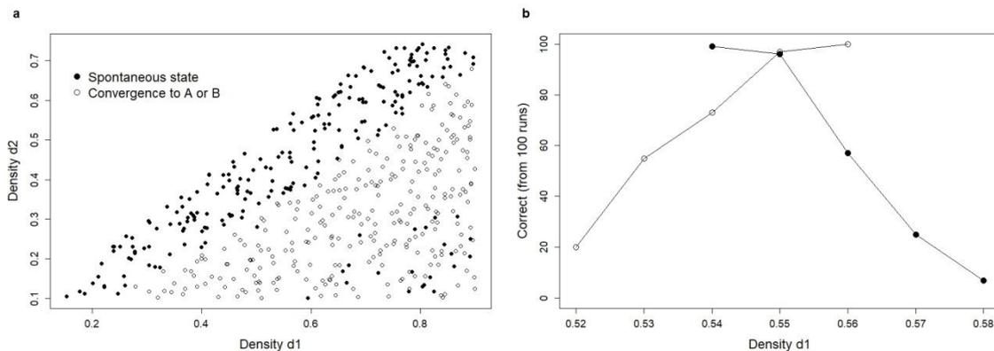
Fig. 5. Decision making in relation to density parameters; a) Monte Carlo analysis based on 500 model runs with no inputs; b) correct responses for varying density parameter  $d_1$  ( $d_2 = 0.36$  in all simulations), black dots: spontaneous state with no input, white dots: convergence with input.
